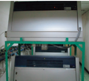
QUV weathering tester
