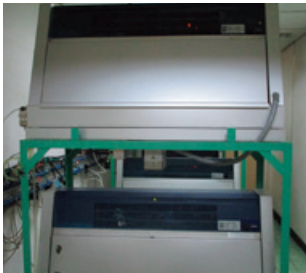
QUV weathering tester
