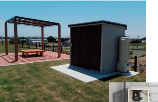
A YODO Monoooki Erumo Storage Shed with a lock that automatically opens after a strong earthquake
