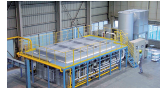
Fire resistance testing unit (horizontal furnace)
