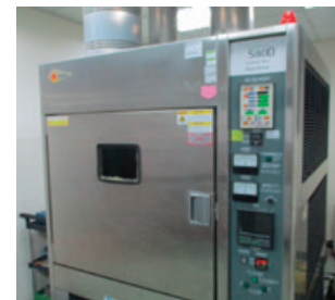
Condensation circulation-type carbon arc weathering tester
