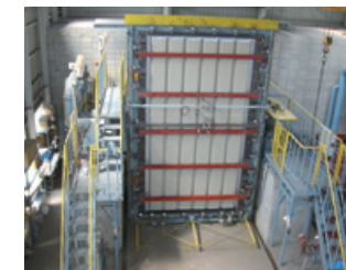
Water seal and wind pressure resistance testing unit
