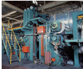
Test calender machine for paper making (gloss finish)
