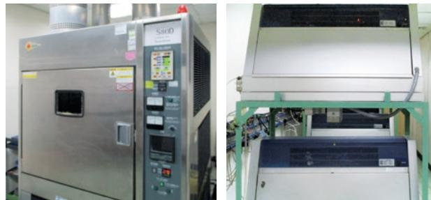
Condensation circulation-type carbon arc weathering tester QUV weathering tester
