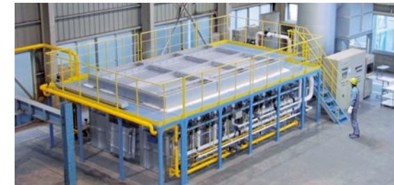
Fire-proof and Fire-resistance Test Equipment (Osaka Plant)
