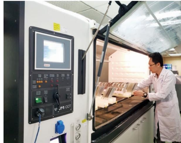
Cyclic corrosion tester (CCT)
