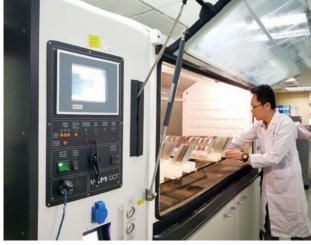
Cyclic corrosion tester (CCT)
